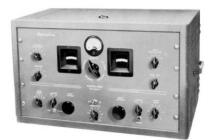
The transmitter power supplies had to be improved. Former electric company telephone pole transformers were obtained and removed from their oil filled housings. These transformers were then used in reverse, with the secondary windings on the transformers used to input 120 or 240 volts into the secondary winding and in turn producing 1,200 or 2,400 volts out of the original primary of the transformers.
